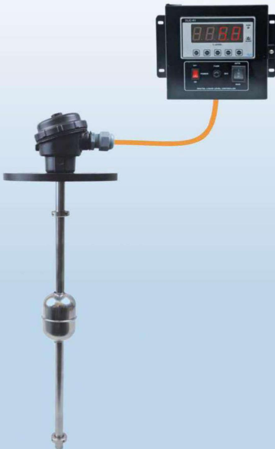
Percentage Level Indicator is used to know the level of liquid in storage or process tank. The unit consist of a Percentage Level Sensor mounted inside the tank & a Digital Level Indicator mounted in control room or pump room or user accessible area.
